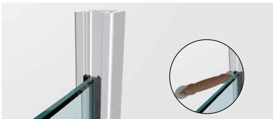
Fit glass retaining rubber (Roller assisted, spray soapy water as lubricant).
