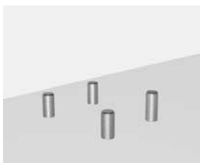
Drill holes & fit the rods.
