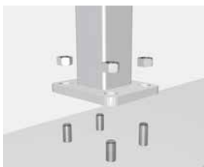
Tighten nuts to fit the posts.
