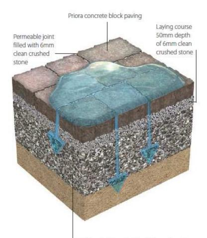
Sub-base 200mm depth of 20mm clean crushed stone with well defined edges
