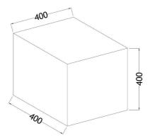
Fill hole with water and allow to drain away naturally. Repeat this process 3 times. If the water does not drain away at all then the sub-grade soil does not have adequate permeability properties
